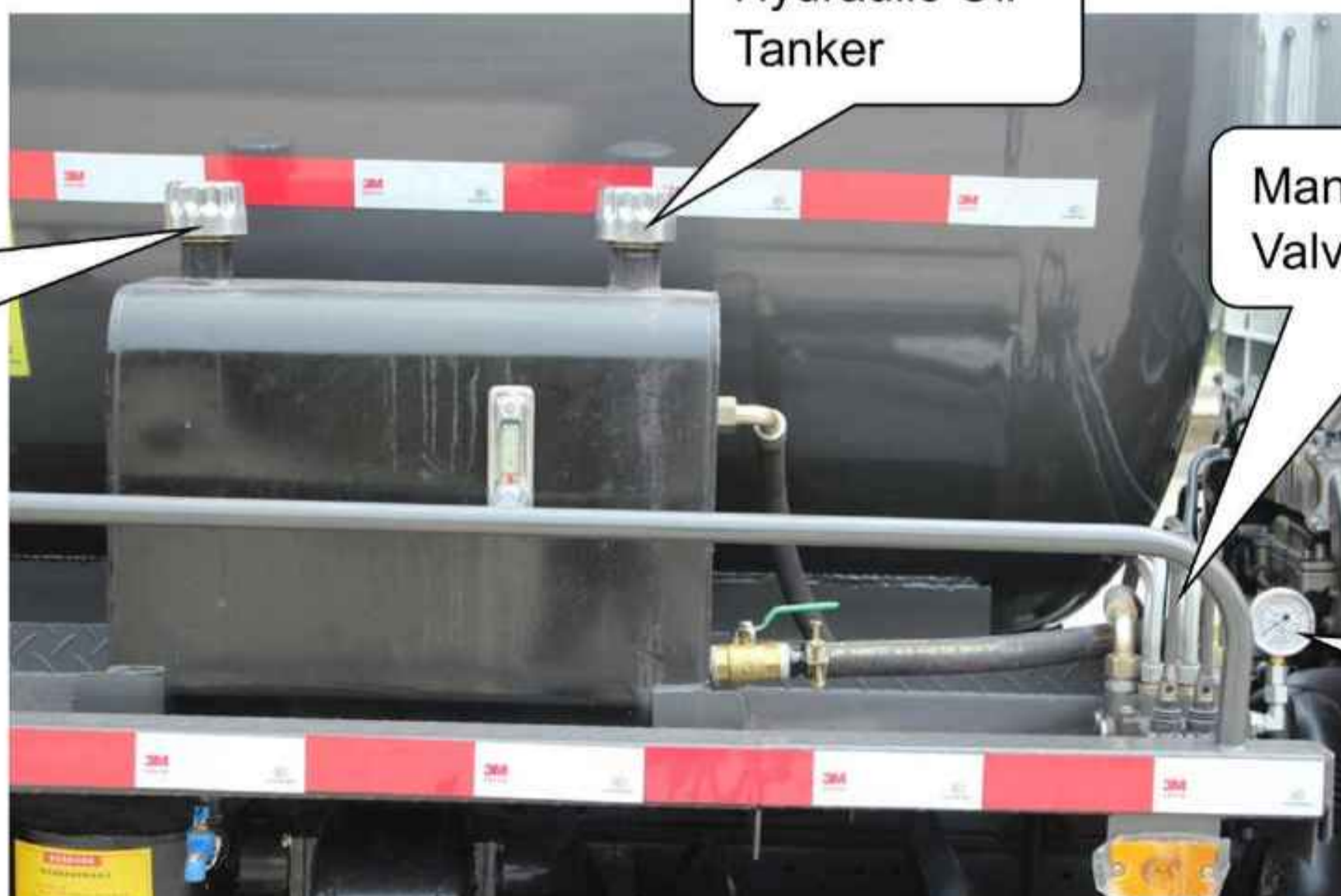
Manual Operated Valve: equipped at side of the platform, which control the vacuum tank rise / fall, and rear door open / close.
